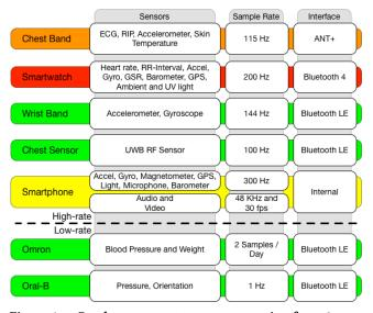
Figure 4: mCerebrum supports sensors ranging from 2 samples/day to 300 Hz per device including: BLE (green), Bluetooth 4.0 (red), ANT+ (orange), and internal (yellow). Additionally, it support short audio and video clips with a high data rate storage mechanism.
