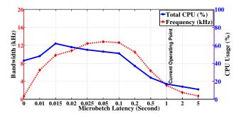
Figure 6: The effect of micro-batch latency on DataKit's communication bandwidth and CPU usage. We observe that with no latency, communication bandwidth is limited by bandwidth limits of IPC, while at higher latency, bandwidth is limited by the buffer size limits of IPC.
