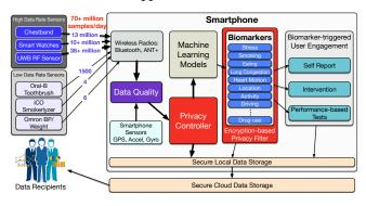
Figure 1: mCerebrum overview illustrating key components such as ingestion of high-frequency sensor data, real-time data quality assessment and biomarker computation.
