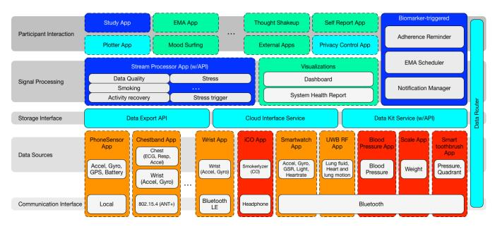
Figure 2: mCerebrum's architecture consists of 5 layers: (1) Communication, (2) Data Sources, (3) Storage, (4) Signal Processing, and (4) Participant Interaction, all connected through a data router. The colors indicate different categorizations of applications – red for high-rate and orange for lower-rate sensors, blue indicates core components of mCerebrum, cyan represents system services, and green represents user-centric applications.
