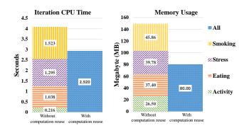
Figure 9: The effects of computation reuse on CPU and memory efficiency. The first columns show the CPU and memory usage when computing four biomarkers without sharing computation. A reduction of 27% CPU time and 47% memory is achieved through reuse, as shown in the second columns.
