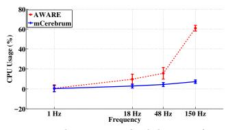
Figure 7: mCerebrum is compared with the AWARE framework by adjusting the total sample rate of the accelerometer, gyroscope, and magnetometers between 18 and 150 hertz per sensor. mCerebrum's benefits by up to 8.4 times lower CPU load when recording at 150 hertz)
