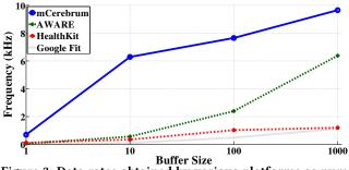
Figure 3: Data rates obtained by various platforms as number of samples (with a common timestamp) are written.
