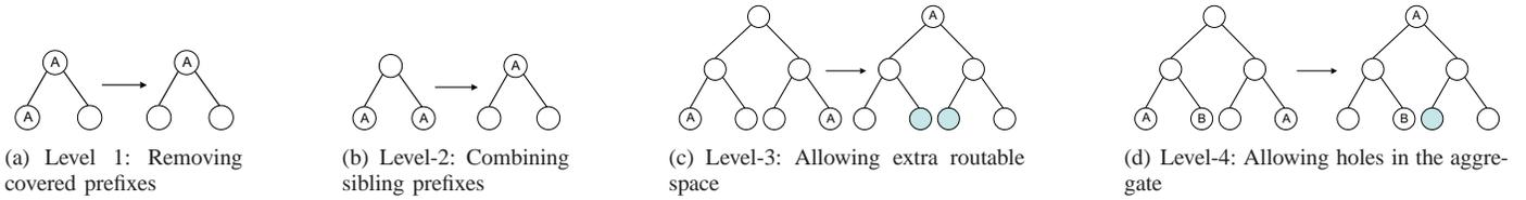
Fig. 2. Different Levels of FIB Aggregation. The binary tree represents part of the IP address space. Nodes labeled with letters are prefixes in the routing table, and the letter represents the next-hop for the prefix. Nodes without labels do not have their corresponding prefixes in the routing table. Filled nodes are extra routable space introduced by the aggregation.
