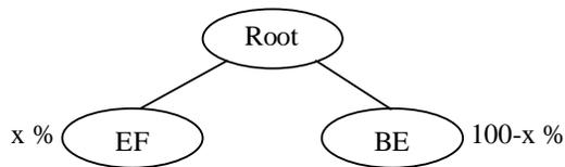
Fig. 4. Allocation of resources at the output interface.
