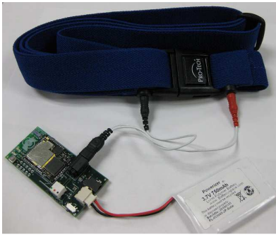
Figure 2: Respiratory Inductive Plethysmograph band (in blue color) and the AutoSense sensor board.
